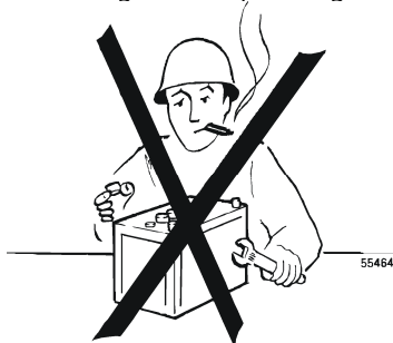
Figure 2 Do not smoke near batteries!
